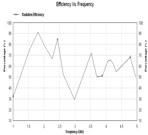
Figure 9(b): Radiation efficiency graph for proposed antenna with changed dimensions.
