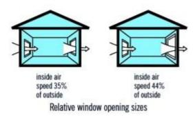
Fig.5 Cross ventilation in doors and windows
