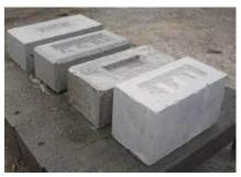
Fig.3 Fly Ash Brick
